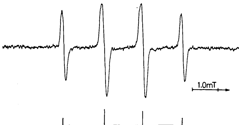
FIGURE 4 ESR spectrum of spin-trapped radicals from UV photolysis of an aqueous solution containing glutathione (100 mM), DMPO (100 mM) and \text{H}_2\text{O}_2 (10 mM). The stick diagram indicates the positions and amplitudes of the hyperfine lines.
